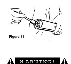
When attaching the driveline yoke to the tractor PTO shaft, it is important that the spring activated locking collar turns freely and that the locking pin is seated on the PTO shaft groove. A loose yoke could slip off and result in personal injury or damage to the mower.
